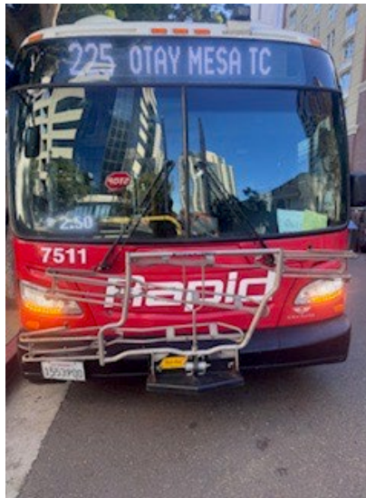
MTS bike rack in the folding position requires grip and upper body strength.
